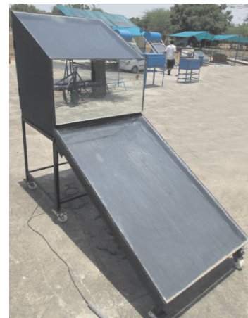
Fig. 5. PCM based Solar Dryer for vegetable and spice crop drying
