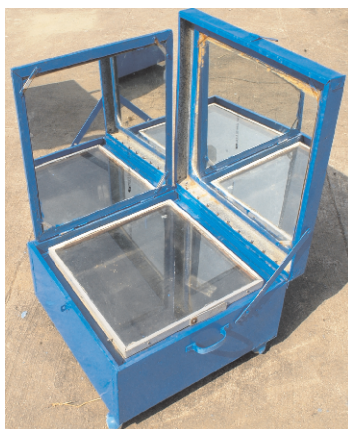
Fig. 7. Box Type Solar Cooker with double reflector
